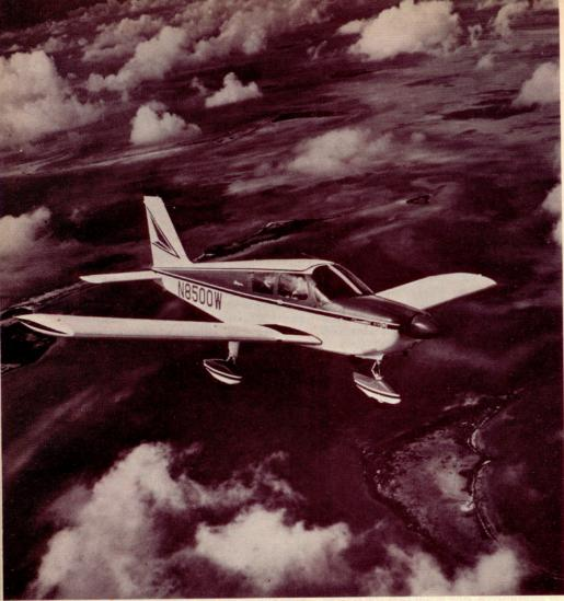
"Super" soundproofing of the cabin and internal dampening of engine mounts enable the new Cherokee 235B to provide an exceptionally quiet and smooth flight. The all-metal 235B has a top speed of 166 m.p.h. and a cruising speed of 156 m.p.h., the manufacturer says. Piper says the low wing, low center of gravity and wide tricycle gear enable the 235B to operate safely on small, unimproved fields
